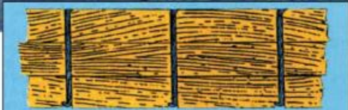
Three 1-1/2" members joined by rivet clinched threaded, 8 gauge, 5" nails.
